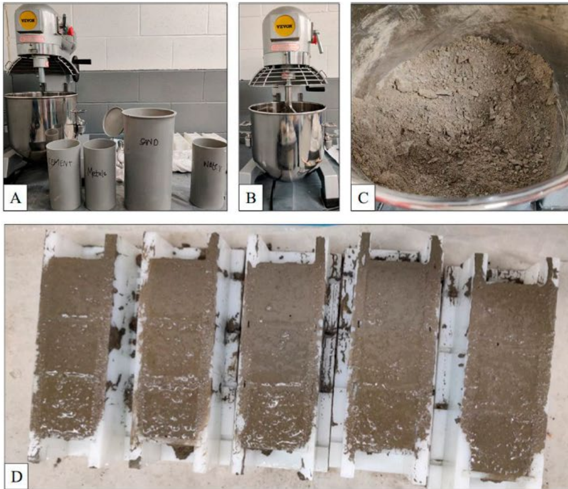
Figure 5. Process of preparing mortar cubes with varied metals: (A) Water, cement, sand, metal mass. (B) Mixing process. (C) Final mix. (D) The 50 mm mortar cubes.
